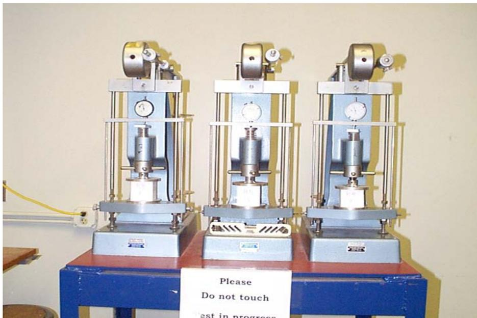
**Photo 1. Creep tests with rear loading cantilever frames**
