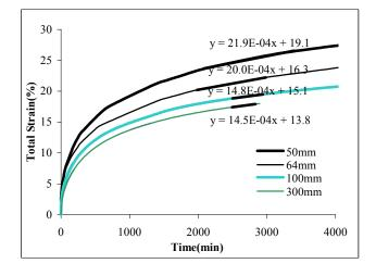
Figure 5. Creep behavior of geofoam of 18 kg/m<sup>3</sup> density at 80% strength
