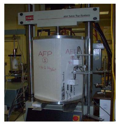
Photo 2. Creep test with hydraulic loading system on a 300 mm x 300 mm x 600 mm geofoam at 30% compressive strength
