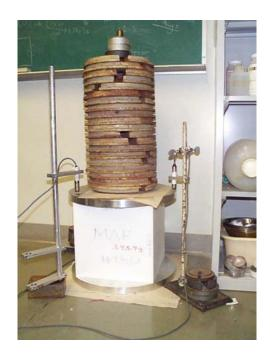
Photo 3. Creep test with dead loading on a 300 mm cube geofoam block at 30% compressive strength
