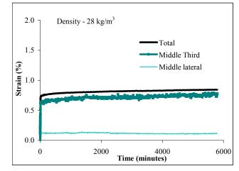
Figure 14. Creep behavior of 300mm cubic sample at 50% strength
