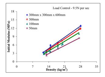
Figure 11. Initial modulus and density for different sample sizes
