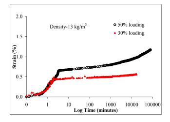
Figure 17. Creep results of 300mm cubic geofoam block tested at 30 and 50 % compressive strength
