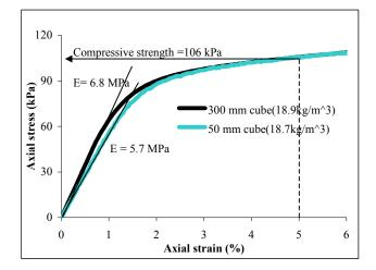
Figure 1. Unconfined compression behavior of EPS geofoam and effect of sample size
