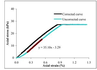
Figure 2. Axial stress vs axial strain for 100mm cube sample of 12.8kg/m<sup>3</sup> density at 50% stress level
