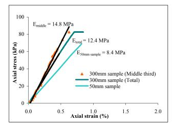
Figure 13. Axial stress vs strain for 300mm cube of 28 kg/m<sup>3</sup> nominal density
