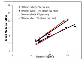
Figure 12. Initial modulus and density for load and displacement controlled tests
