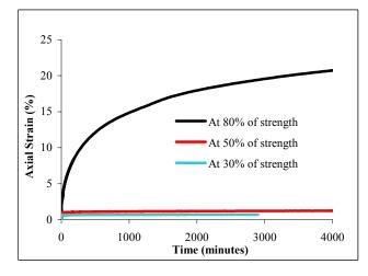
Figure 3. Creep behavior of 100mm cube of 18 kg/m<sup>3</sup> density at different stress levels
