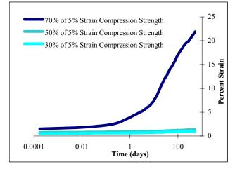
Figure 18. Creep results of 50mm conventional specimens (After Sheeley (2000))
