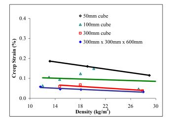
Figure 7. 24 Hour creep strain for samples loaded at 30% strength
