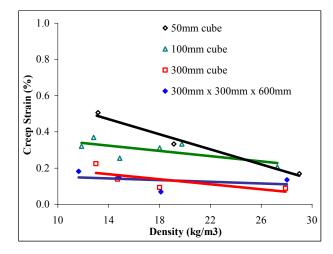
Figure 9. 24 Hour creep strain for samples loaded at 50% strength
