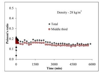
Figure 16. Poisson's ratio for 300mm cube geofoam of 28 kg/m<sup>3</sup> density
